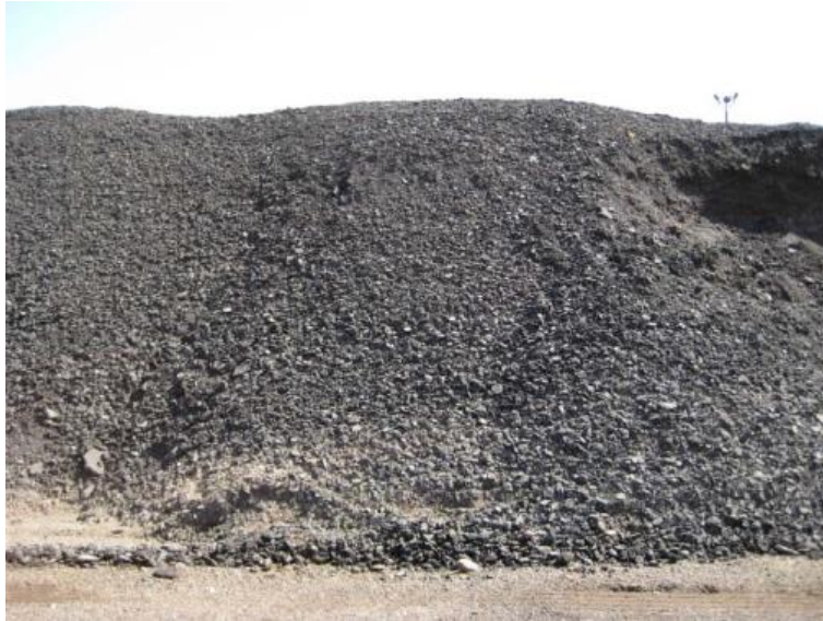
Figura 1. Material de RAP acumulado. (Federal Highway Administration, 2011). Reclaimed Asphalt Pavement in Asphalt Mixtures: State of the Practice, p. 20.
