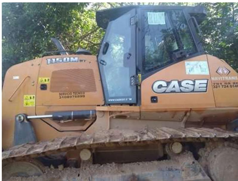
Figura 11. Tractor de oruga 1150M
